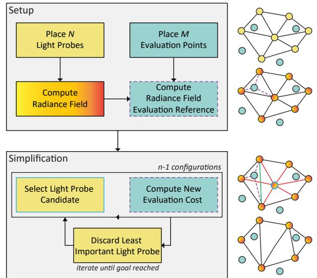
**Figure 2:** Our method consists of two common steps: “Setup” and “Simplification” (left). A simplistic graphical example is also offered to demonstrate the workflow of this approach (right).
